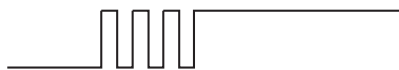
Without a debounce filter, the signal is interpreted to change state multiple times.
