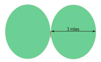
Viewed from the side, however, the radiation pattern of an omni-directional antenna is doughnut shaped.
