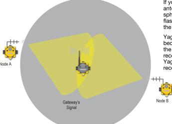
If you compare antenna radiation patterns to light, an omni antenna radiates a radio signal like a light bulb — evenly in a spherical pattern. A directional antenna radiates similar to a flashlight — focusing the signal only in one direction. The higher the gain, the more focused the beam becomes.
