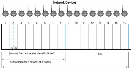
TDMA frame for a network of 16 Nodes
