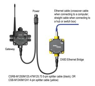
Connect a DX83 Ethernet Bridge to a host system using the industrial Ethernet connection on the DX83. To connect the DX83 directly to the host system without using an Ethernet switchbox/hub, some host systems may require a crossover cable.
