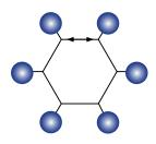
**Pros**—The signal can reverse direction when a link fails.
