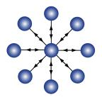
**Pros**—The gateway maintains a communications connection with each node on a separate communications path; if communication between one node and the gateway fails, the rest of the network is unaffected; and chattering nodes are removed from the network.
