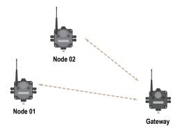
In our simple example, a sensor wired to Node 1 is an input device connected to Node 1's input. Data is transmitted to Node 2 and a device connected to Node 2's output performs a task, for example, turning on a light.
