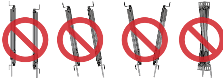
Figure 26. Incorrect Sensor Alignment
