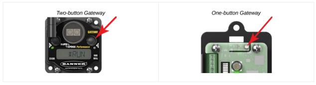
The LEDs flash alternately when the Gateway is in binding mode. Any Node entering binding mode will bind to this Gateway.
