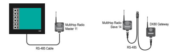
Banner's MultiHop radios and Gateways use non-isolated RS-485 circuits and must have their grounds connected.
