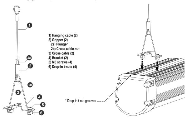
When feeding the cable through the gripper, allow at least one inch of cable beyond the gripper. Do not feed any excess cable into the light housing. To adjust the gripper position:
