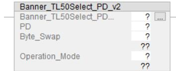
2. In the AOI, right-click on the question mark on the line labeled “Banner\_TL50Select\_PD\_v2”. Click New Tag. Name the new tag. This example uses the name “TL50Select\_IOLM2\_04\_PD\_Status”. The example naming convention accounts for this being an TL50 Pro Select device connected to IO-Link Master #2, port #4, in our program. More masters could be named IOLM1, IOLM3, and different sensors could be connected at other port numbers, etc.
