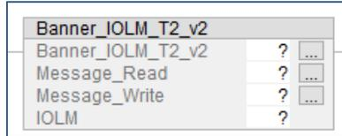
2. In the AOI, right-click on the question mark on the line labeled “Banner\_IOLM\_T2\_v2”. Click New Tag. In this example, we’ll use the name “IOLM2\_Status”. The example naming convention accounts for this being the #2 IO-Link Master in our program. More masters could be named IOLM1, IOLM3, etc.
