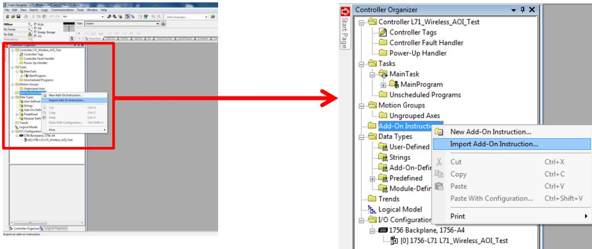
3. Navigate to the correct file location and select the AOI to be installed. In this example the "Banner\_TL50Select\_PD\_v2.L5X" file will be selected. Click the Open button.
