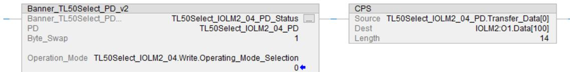
If a Banner IO-Link Master is being used, setup a Move block. Send a 1 to the Activate Outputs array value (see table for each port’s value). As an example, if port 1 needs the process data outputs active then send a 1 to 181.
