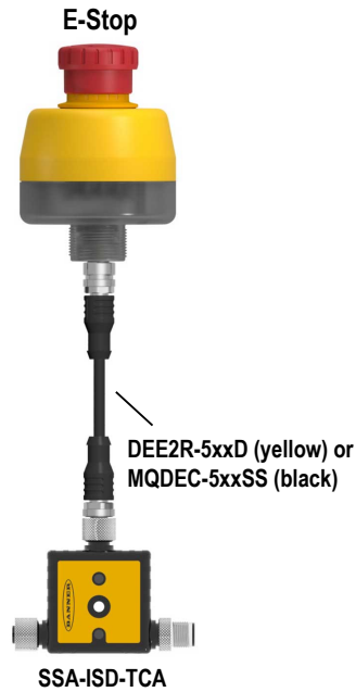
Wiring the SSA-ISD Connect to an SSA-EB1P-02ECQ5A E-stop button with a MQDEC-5xxSS cordset
