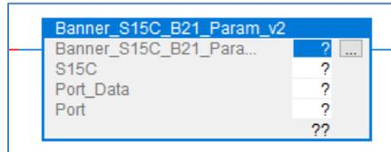
2. In the AOI, right-click on the question mark on the line labeled “Banner\_S15C\_B21\_Param\_v2”. Click New Tag. In this example, we’ll use the name “S15C\_B21\_IOLM1\_01\_Status”. The example naming convention accounts for this being a S15C sensor connected to IO-Link Master #1, port #1, in our program. More masters could be named IOLM2, IOLM3, and different sensors could be connected at other port numbers, etc.
