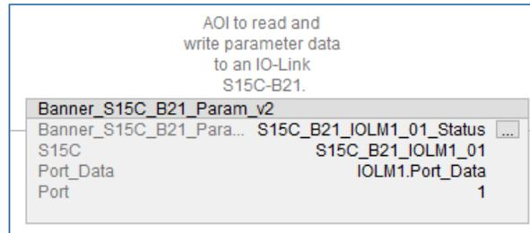
3. Add an Examine On instruction before the S15C B21 AOI on the same ladder rung and tie it to the IO-Link Master AOI’s “Port\_Activate” bit corresponding to the port number to which the S15C device is connected. In this example the S15C-B21 is on port 1 of the IO-Link Master named IOLM1, so the bit “IOLM1.Port\_Data.Port\_Activate.1” is used.
