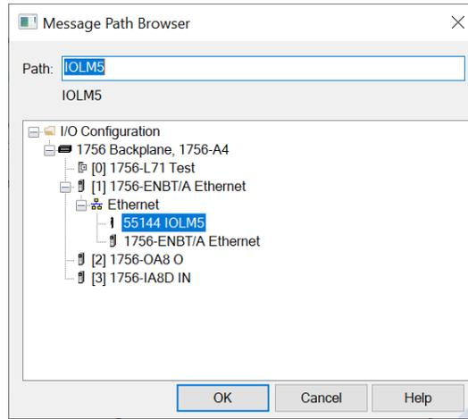
12. Now configure “Message\_Write”, setting up the Explicit Message that will handle the other half of the communications between the PLC and the IO-Link Master. Click on the “...” button at the far right of the “Message\_Write” line.
