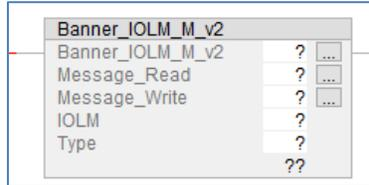
2. In the AOI, right-click on the question mark on the line labeled “Banner\_IOLM\_M\_v2”. Click New Tag. In this example, we’ll use the name “IOLM5\_Status”. The example naming convention accounts for this being the #5 IO-Link Master in our program. More masters could be named IOLM1, IOLM2, etc.
