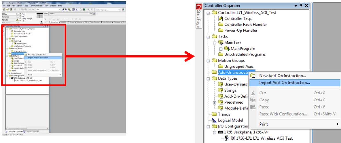
3. Navigate to the correct file location and select the AOI to be installed. In this example the "Banner\_IOLM\_C\_v2.L5X" file will be selected. Click the Open button.
