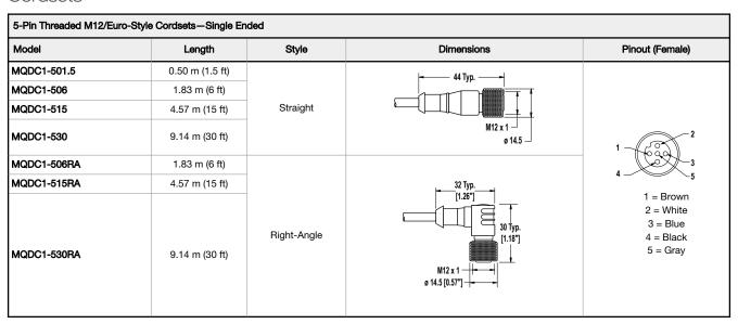
All measurements are listed in millimeters [inches], unless noted otherwise.
