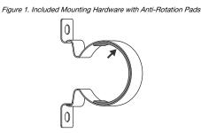
Note: When using the optional mounting hardware, cut the anti-rotation pad and apply it to both sides of the mounting bracket as shown.
