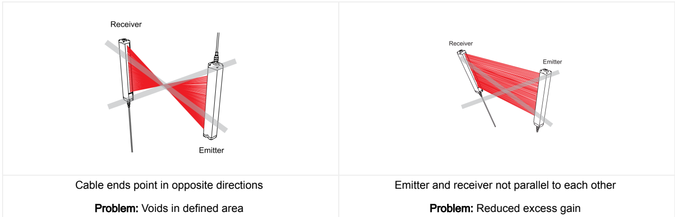
Figure 9. Examples of Incorrect Emitter/Receiver Orientation
