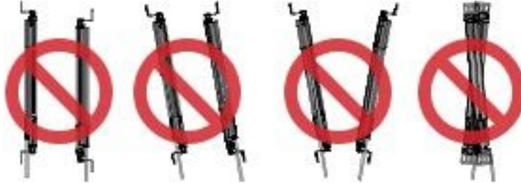
Figure 23. Incorrect Sensor Alignment
