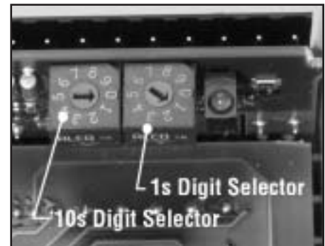
Figure 5. MAC ID address rotary selectors and LED
