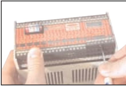
Figure 10. Gently pry up each of the five wiring barriers.
