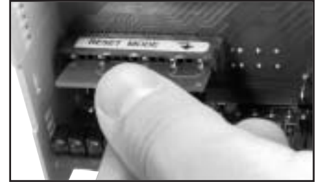
Figure 6. Selecting Auto or Manual Reset
