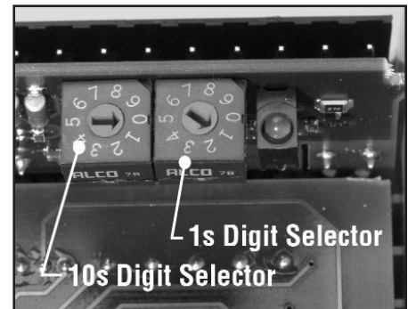
Figure 5. MAC ID address rotary selectors and LED
