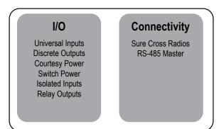
Inputs/Outputs—On-board universal and programmable I/O ports connect to local sensors, indicators, and control equipment.
