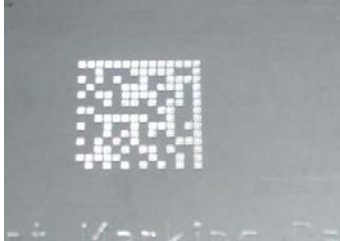
Figure 230. Directly Marked Dot Matrix Code Characterized by Outstanding Separation Distance between Adjacent Code Elements
