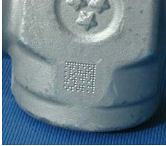
Figure 229. Dot Peening Marking on Metal Surface with Multi-dot per Code Element
