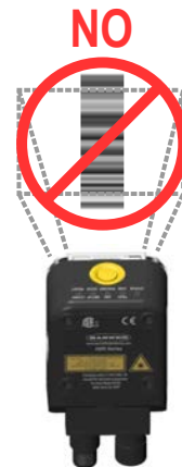
Figure 14. Code Out of FOV Due to Tilt Angle
