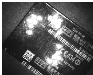
Figure 245. Example B: Good Illumination on Left Code
