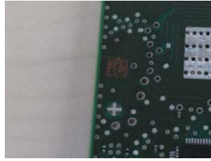
Figure 280. Multicolored DPM - Peripheral Group ALL Sectors On: Incorrect Illumination
