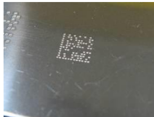
Figure 276. Multicolored DPM - Peripheral Group: Good Illumination
