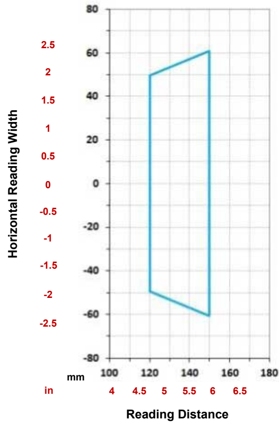
Figure 206. Data Matrix 0.19 mm (7.5 mils)
