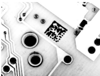
Figure 232. Data Matrix Code Directly Marked on PCB Surface by Using Laser Etching Technology
