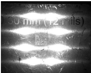
Figure 283. Red: Incorrect Illumination
