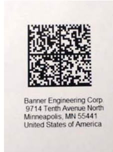
Figure 224. Address Coded in Data Matrix Symbology for Automated Mail Processing
