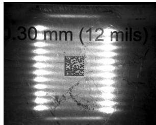
Figure 286. Multicolored DPM - Peripheral Group Left and Right Sectors ON: Good Illumination
