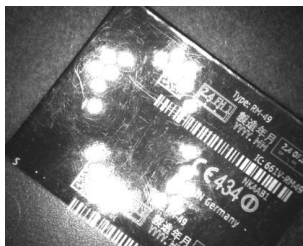
Figure 244. Example A: Incorrect Illumination
