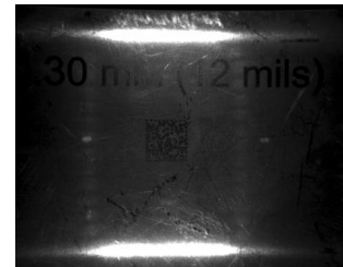
Figure 285. Multicolored DPM - Peripheral Group Top and Bottom Sectors On: Incorrect Illumination
