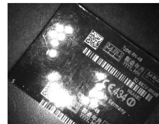
Figure 246. Example C: Good Illumination on Right Code
