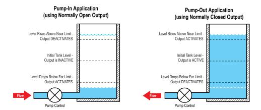
The **HIGH/LOW** mode (switch #2 ON) provides the switching logic required for fill-level, web tensioning control, and similar applications. In the HIGH/LOW mode, the output energizes when the target reaches the first sensing window limit, and stays energized until the target moves to the second limit. The output then de-energizes at the second limit and does not re-energize until the target moves, again, to the first limit.
