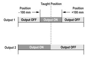
Figure 7. Using simultaneous auto-window/background suppression (normally open illustrated)
