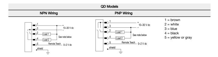
NPN or PNP hookup must agree with DIP-switch settings. Banner Engineering Corp. recommends connecting the shield wire to earth ground or DC common.
