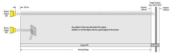
Figure 6. An application for Auto-Window feature (retroreflective mode)
