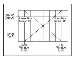
Figure 5. Output Slope
