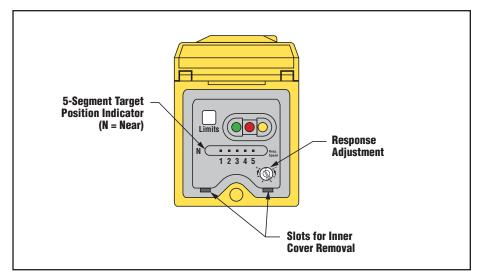
Figure 1. Analog Q45U (45LMA card) features
