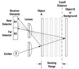
Object is sensed if amount of light at R1 is greater than the amount of light at R2 Figure 1. Fixed-field concept
