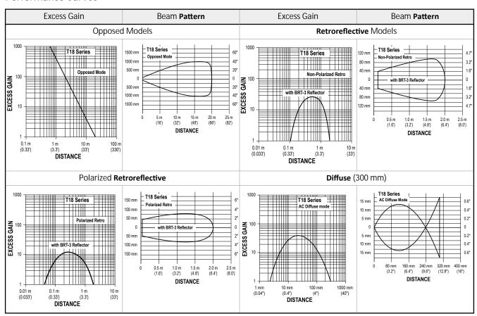
For the polarized retroreflective and retroreflective models, the performance is based on a model BRT-3 retroreflector (3 in diameter). The actual sensing range may be more or less than specified, depending on the efficiency and reflective area of the retroreflector used. For the diffuse models, the performance is based on a 90% reflectance white test card.
