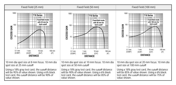
For the fixed field models, the performance is based on a 90% reflectance white test card. Focus and spot sizes are typical.
