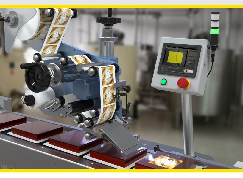
Banner Engineering offers a wide variety of industrial automation components that are ideal for use on labelling equipment including safety, indication and sensors. The SLE5 High Speed Optical Label Sensor was designed to reliably detect either labels or their backing. The simple, one-button TEACH mode provides fast sensor commissioning, and the dovetail design facilitates tool-less installation directly on the dispensing ledge.
