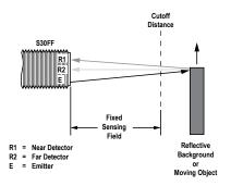
A reflective background object in this position or moving across the sensor face in this axis and direction may cause false sensor response.
