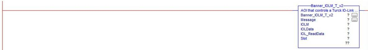
2. In the AOI, right-click on the question mark on the line labeled “Banner\_IOLM\_T\_v2”. Click New Tag. In this example, we’ll use the name “IOLM4\_Status”. The example naming convention accounts for this being the #4 IO-Link Master in our program. More masters could be named IOLM1, IOLM3, etc.
