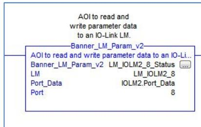
3. The LM AOI is now linked to the IO-Link Master AOI. Add an Examine On instruction to the beginning of the ladder rung and tie it to the IO-Link Master AOI’s “Port\_Activate” bit corresponding to the port number to which the LM is connected. In this example the LM is on port 8 of the IO-Link Master named IOLM2, so the bit “IOLM2.Port\_Data.Port\_Activate.8” is used.
