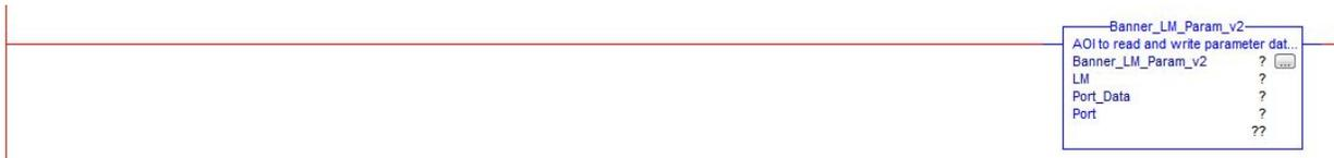
2. In the AOI, right-click on the question mark on the line labeled “Banner\_LM\_Param\_v2”. Click New Tag. In this example, we’ll use the name “LM\_IOLM2\_8\_Status”. The example naming convention accounts for this being a LM device connected to IO-Link Master #2, port #8, in our program. More masters could be named IOLM1, IOLM3, and different sensors could be connected at other port numbers, etc.
