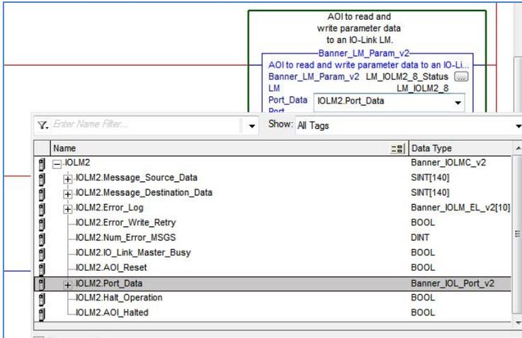
2. For the last line of the LM AOI, “Port\_Number”, type in a number equal to the IO-Link Master port number to which the LM is connected. In this example, the LM is on port 8.
