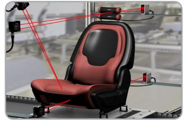
A pair of L-GAGE® LE550 laser triangulation sensors measure the forward and rearward movement of a vehicle seating system as part of a series of inspections verifying range of movement
