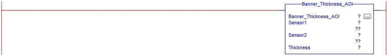
2. In the AOI, right-click on the question mark on the line labeled “Banner\_Thickness\_AOI”. Click New Tag. Name the new tag. This example uses the name “Thickness\_1\_Status”. The example naming convention accounts for this being the first thickness measurement in the system. Click create.
